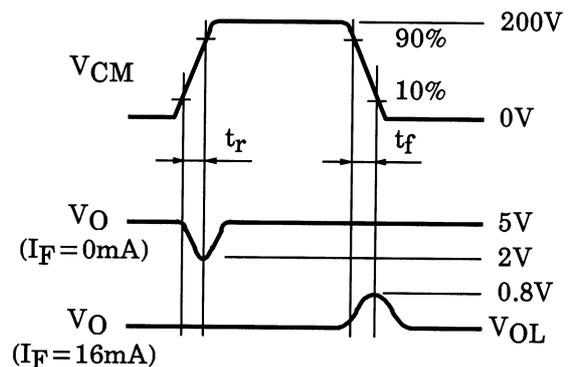
$$CM_H = \frac{160(V)}{t_r(\mu s)}, \quad CM_L = \frac{160(V)}{t_f(\mu s)}$$
